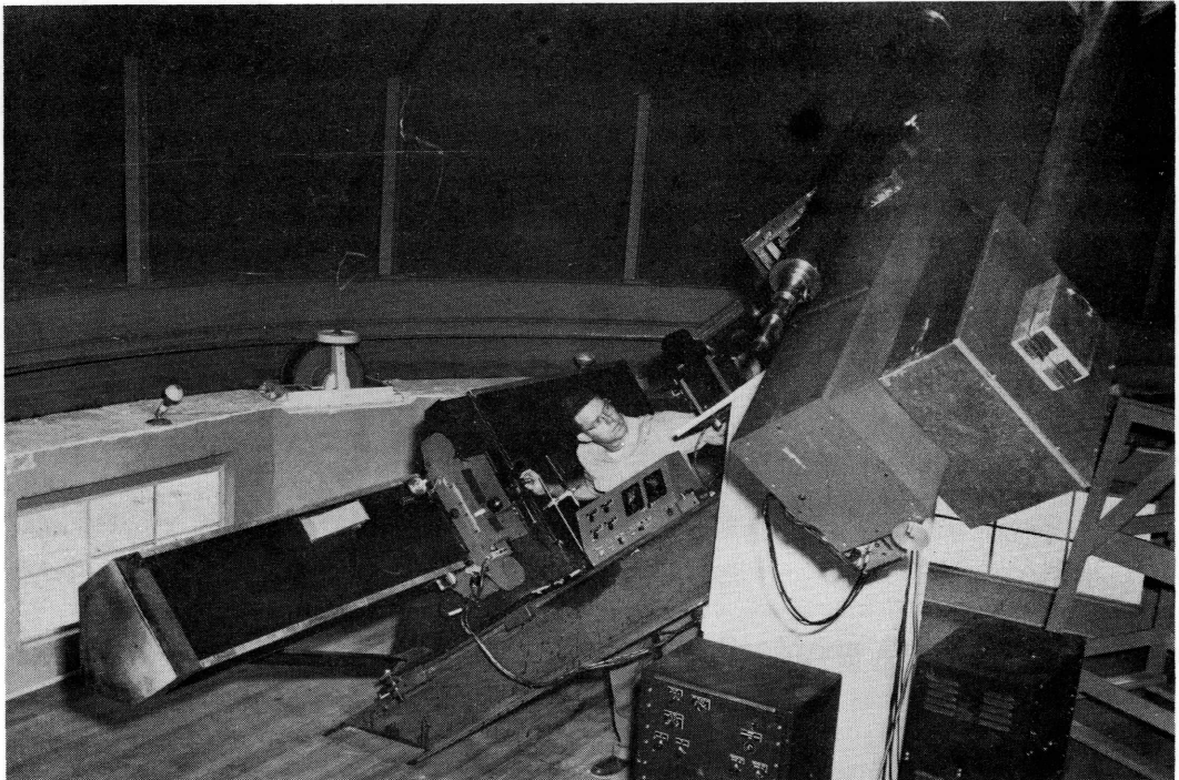
The new 5-inch patrol coronagraph and spectrograph at Climax. Mr. Keith Watson, Climax observer, shown at the controls of the all-reflection spectrograph and automatic scanning slit mechanism.
