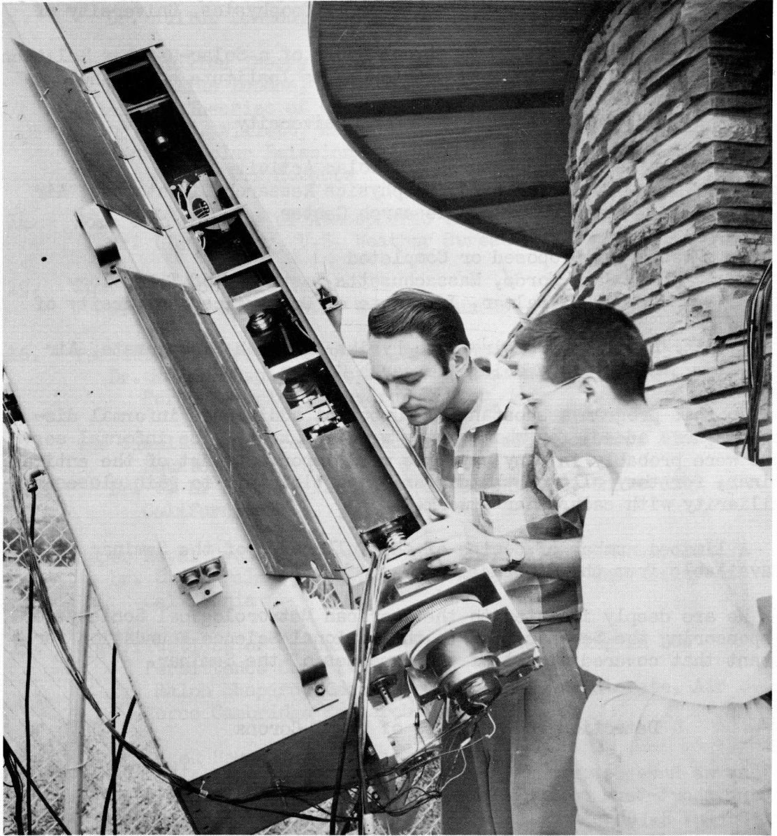
Figure 2 Axtell (left) and Wlérick (right) are shown here checking the operation of the K-coronameter outside the Sommers Bausch Observatory in Boulder. Immediately above Axtell's hand is the Lallemand multiplier photocell that detects the light from the electron corona. It gives a signal that is graphically recorded on an Esterline-Angus recorder located inside the building.
