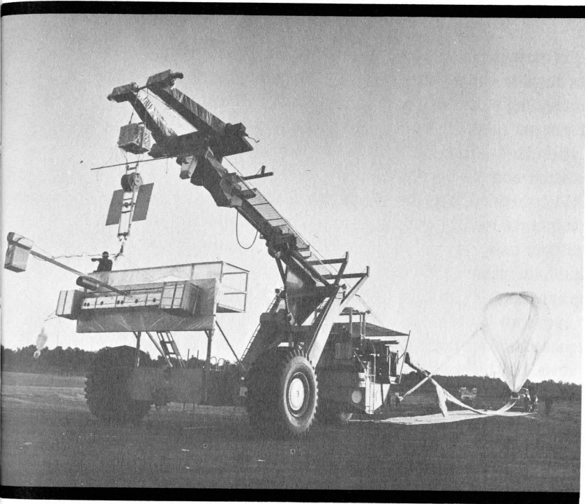
At NCAR's scientific balloon launch station at Palestine, Texas, a balloon is readied for launch. The launch vehicle, known as "Tiny Tim," is able to support heavy, fragile payloads until they are safely airborne.
