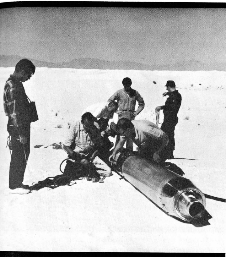
ENCAR-1 landed on a dune after its successful flight. A recovery party arrived at the scene within an hour. The sampler was essentially undamaged and will be reused.
