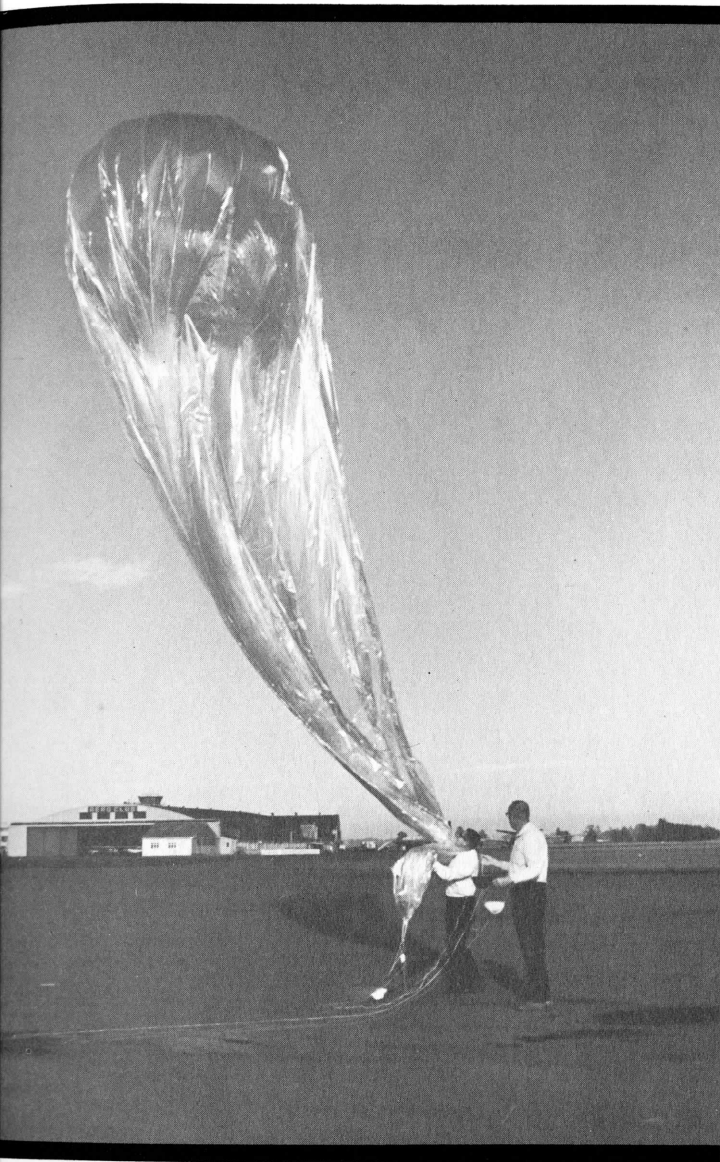
A constant-level GHOST balloon is launched from Christchurch, New Zealand. Balloons such as these, drifting with the wind, will transmit temperature, pressure, and wind data to satellites for relay to ground stations.
