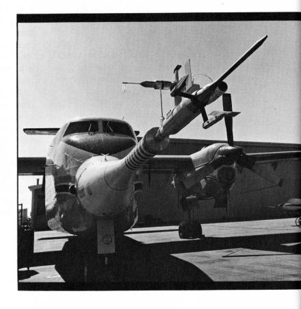
A new airborne turbulence measuring system is mounted on a nose boom installed on NCAR's Buffalo aircraft. The base of the boom contains an inertially stabilized reference platform which precisely determines motions of the aircraft from the moment of takeoff. The system is the most accurate of its kind and will be an asset to a variety of studies on the motions and transfers of energy in the atmosphere.
