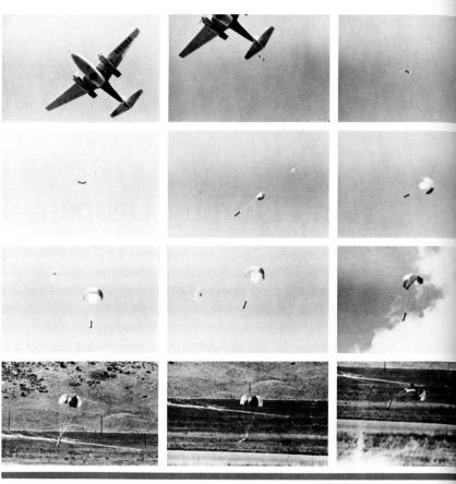
A prototype wind-finding dropsonde is released from Colorado State University's research aircraft. The dropsonde, shown in the lower photograph, weighs only 1.75 kilograms (3.8 pounds). Since these sondes are to be used over ocean areas, they will be expendable, built of relatively inexpensive materials comparable to those used in conventional radiosondes.
